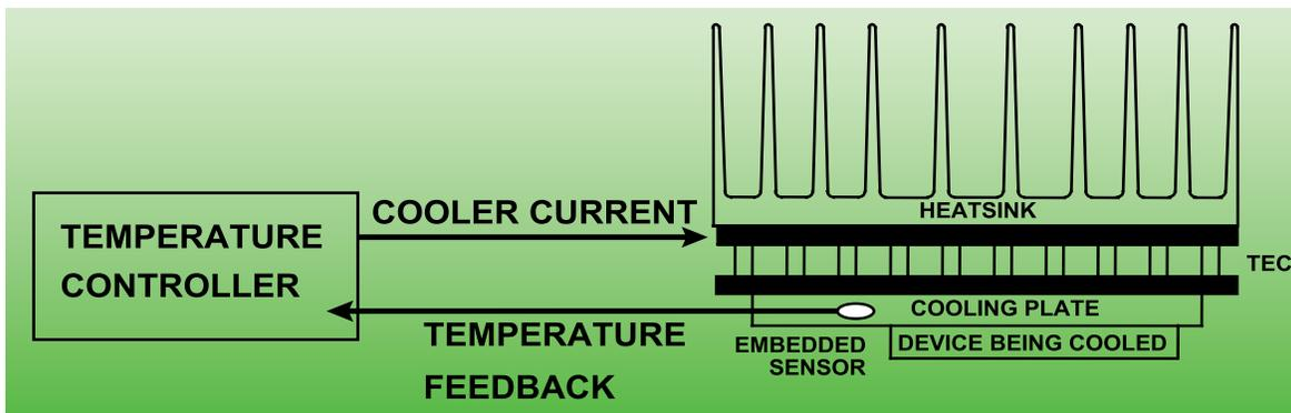
Figure 1. A simple thermoelectric control system uses feedback from a temperature sensor to maintain a device at constant temperature.
