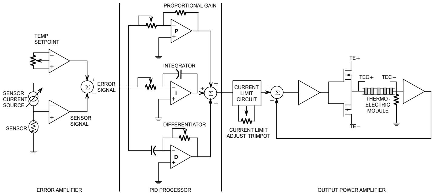
**Figure 2. PID Loop Containing Error Amplifier, Power Output Amplifier and PID Processor**
