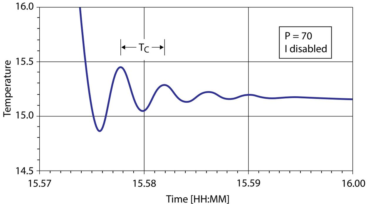
**Figure 4. Find the critical proportional gain ( $k_c$ ) necessary to cause the temperature to begin damped oscillations. The oscillation period is  $T_c$ .**
