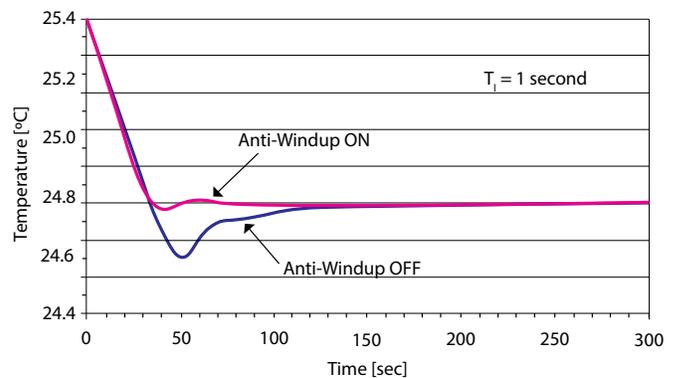
**Figure 6. Comparison of response with and without anti-windup**
