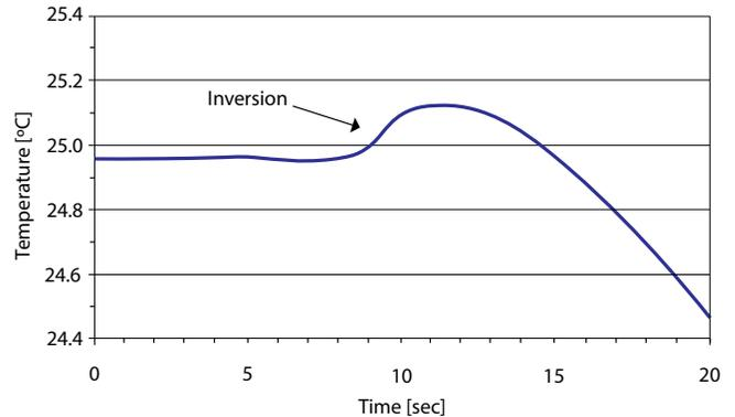
**Figure 5. Inversion is the term for the system initially responding in the opposite direction from that commanded by the control signal.**
