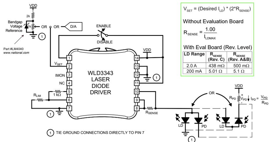
**Figure 8. Type C Laser Diode with WLD3343 in Constant Current Mode**
