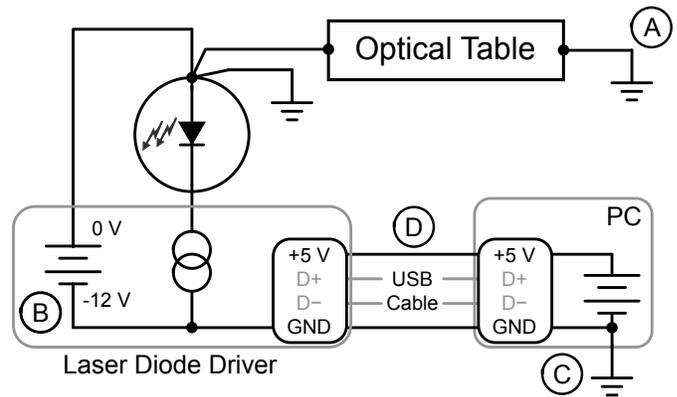
**Figure 10. Example Configuration with USB Control**
