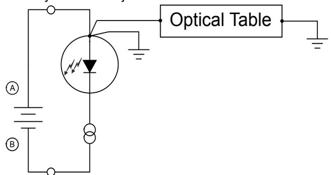
**Figure 4. Earth-Grounded Anode**
