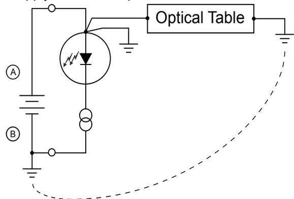
**Figure 5. Problem: Grounded Anode & Power Supply**
