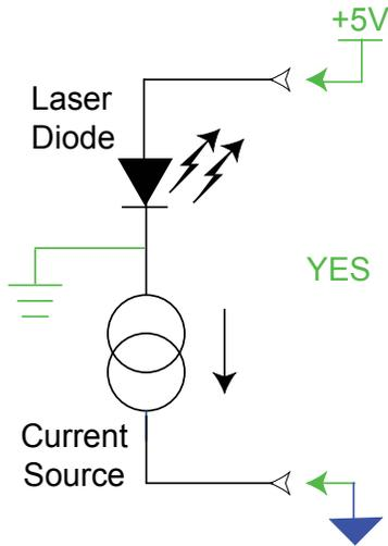
**Figure 9. Floating Power Supply**
