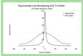
Driving the QCL with a low-noise laser diode driver and integrating over a suitable time period results in a laser linewidth of approximately 40 MHz. Switching to the ultra-low noise QCL driver, and making other improvements in the electronics, narrows the spread to 300 kHz.
