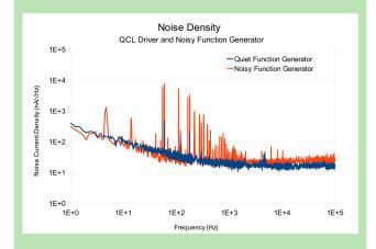
Modulating the current with a low-noise function generator dramatically reduces noise density and cumulative noise, and suggests that additional effort with the function generator will yield further improvements.
