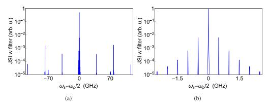
**Fig. 6.** Theoretical two photon JSI from CE-SPDC after the FP filter. Graphs as in Fig. 4, but  $|\phi_{\rm filt}(\omega_s,\omega_p-\omega_s)|^2$  is shown. This describes the JSI when the filter, described in subsection 3.3, is placed in the signal arm and no filter in the idler arm (so that  $|T_i|=1$ ). The contribution of unwanted photons is 2.3 % within a window  $\pm 1$  nm when the filter is set to transmit the brightest mode from the CE-SPDC.
