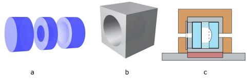
**Fig. 5.** FP filter assembly. (a) The FP filter consisting of one concave mirror, an annular spacer, and a plano mirror in face-to-face contact is housed in a (b) hollowed aluminum block and cemented around the edges with epoxy. (c) Vertical cross section of the filter assembly: aluminum box and heat sink are shown in grey, the Peltier element in red, the mirrors and spacer in shades of blue and the insulator in orange.
