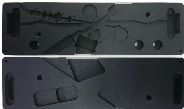
**Fig. 1.** Photographs of the laser photometer base plate (upper), and lid (lower). The parts were CNC milled from aluminium, and then anodized, by separate contract manufacturing organisations.
