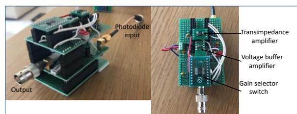
**Fig. 3.** Optical detection setup and circuit assembly (plan view).
