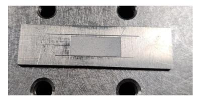
Figure 4.2.13: Stainless-steel substrate.
