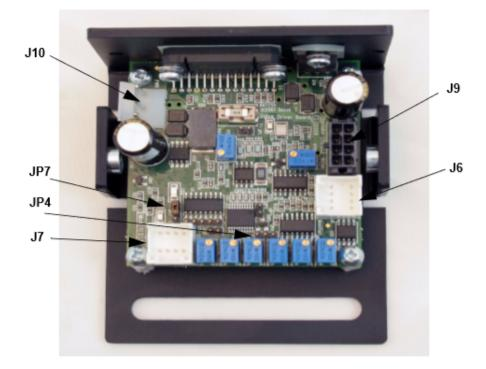
Figure 4.1.11: Driver board of GVS001 Thorlabs [3].
