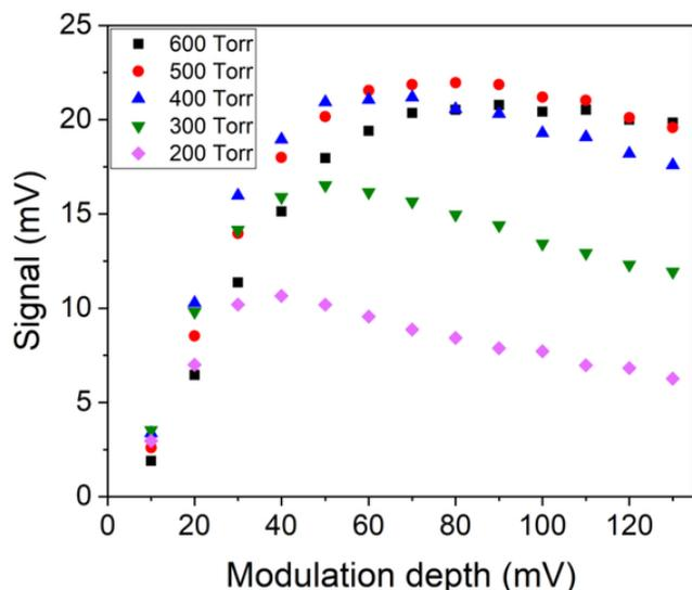
**Figure 5.** QEPAS signal of a certified 500 ppm CO:SF<sub>6</sub> mixture, as a function of the modulation depth set on the waveform generator. Operating pressure varied from 200 Torr to 600 Torr.<sup>1</sup>
