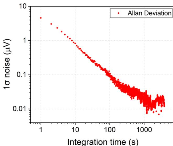
**Figure 7.** 1σ noise of QEPAS signal as a function of the lock-in integration time as result of Allan-Werle deviation analysis.<sup>1</sup>
