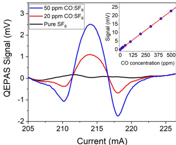
**Figure 6.** QEPAS signals acquired at different concentrations of CO in SF<sub>6</sub> mixture and QEPAS signal of pure SF<sub>6</sub> as a function of the laser injection current. (inset) CO peak signals acquired at different CO concentrations (blue dots) and the corresponding linear fit (red line).<sup>1</sup>
