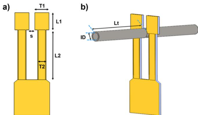
**Figure 3. (a) Schematic diagram of the T-shaped grooved QTF, with geometrical parameters. T1 = 2.0 mm; T2 = 1.2 mm; L1 = 2.4 mm; L2 = 7.0 mm; s = 0.8 mm. Carved grooves on the QTF prong are 50 μm deep. (b) Schematic diagram of the QEPAS spectrophone.<sup>1</sup>**
