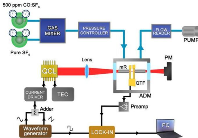
**Figure 4. Schematic of the QEPAS sensor for CO detection in the SF<sub>6</sub> matrix. TEC, thermo-electric cooler; ADM, acoustic detection module; PM, power meter; DAQ, data acquisition; PC, personal computer.<sup>1</sup>**
