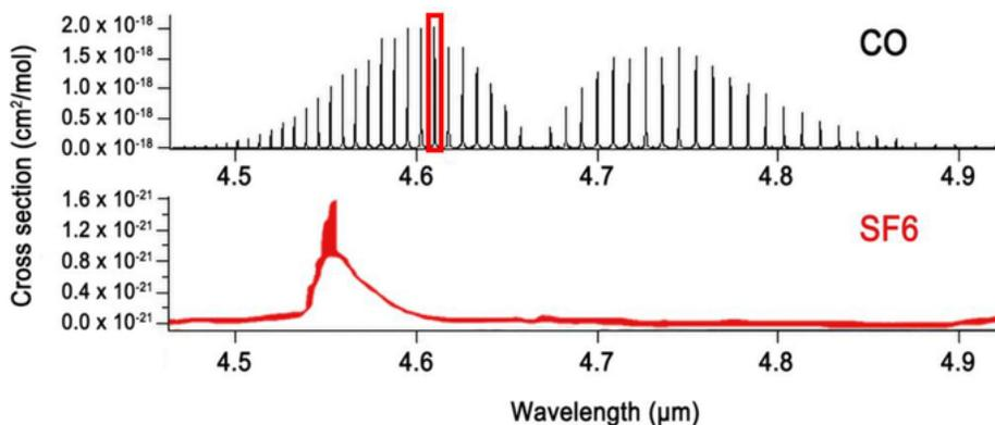
**Figure 2.** CO absorption cross section (black line) and SF<sub>6</sub> absorption cross section (red line) simulated using PNNL database. The red rectangle points at the CO feature targeted for the detection.<sup>1</sup>
