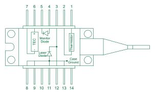
Figure 9. Standard Type 2 Laser Diode Butterfly Schematic
