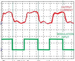
Figure 14. 20 kHz Square Wave, 4-foot twisted wires
