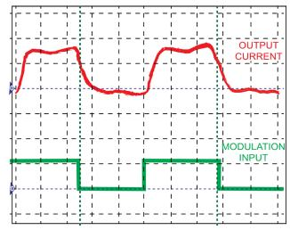
Figure 16. 20 kHz Square Wave, Filtered, Untwisted Wires
