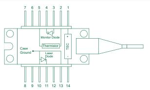
Figure 8. Standard Type 1 Laser Diode Butterfly Schematic
