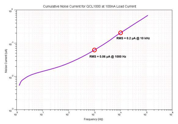
Figure 6. RMS noise - Integration of data from Figure 5 QCL1000 with shorter cable and minimal AC interference
