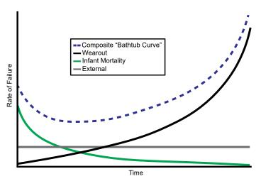
Figure 17. Laser Rate of Failure vs. Time
