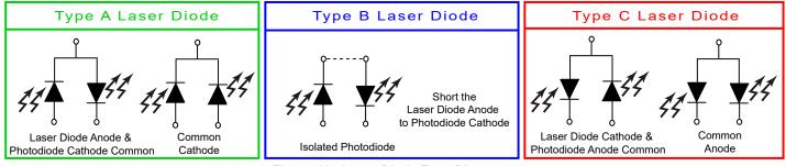
Figure 10. Laser Diode Type Diagrams
