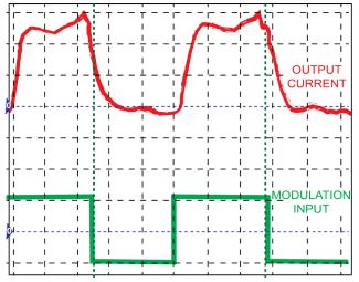
Figure 13. 20 kHz Square Wave, Negative Bias
