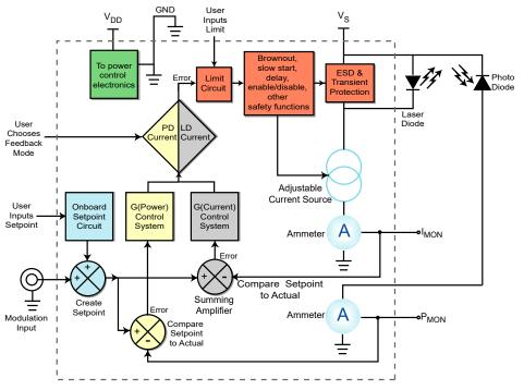
Figure 1. Laser Diode Driver Block Diagram
