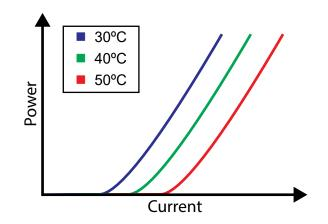
Figure 3. Output Power vs. Input Current with Multiple Temperatures
