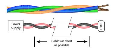
Figure 4. Twisted wires (top) and short, twisted wires from a supply to the load (bottom)
