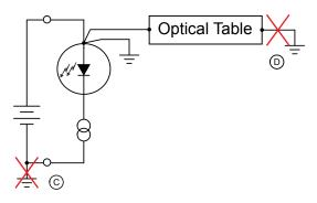
Figure 6. Solution: Break the Ground Short at One Point (C or D)
