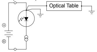
Figure 4. Earth-Grounded Anode
