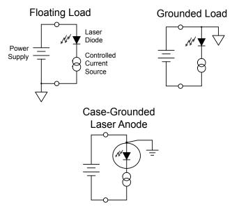
Figure 2. Three Typical Grounding Configurations
