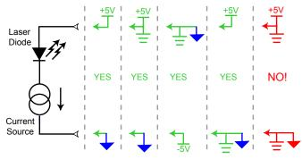
Figure 3. Example Grounding Configurations
