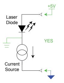
Figure 9. Floating Power Supply
