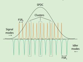
Figure 2. Cluster effect. The longitudinal modes for signal are shown in orange and the modes for idler are in green. The two arrows indicate the direction in which frequency increases. The overlap condition is periodical, but because of the difference in the FSRs for signal and idler, the modes that are next to the fully overlapping ones coincide only partially. This leads to a spectrum that is made of clusters of modes, separated by  $\Delta v_c$ .<sup>1</sup>
