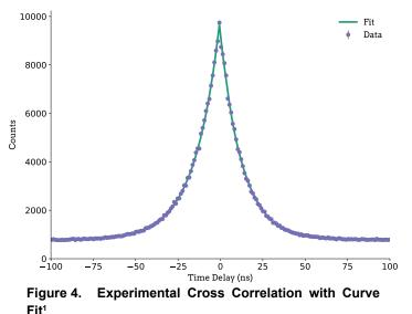
From the data, the effective bandwidth of the photons is found to be  $10.9 \pm 0.3$  MHz for the photon pairs. This is close to the few megahertz linewidth of typical atomic transitions.
