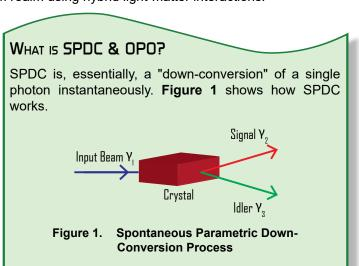
One photon ( $\gamma_1$ ) enters the nonlinear crystal and is down-converted into two separate photons: signal and idler ( $\gamma_2$  and  $\gamma_3$ ). Down-converted means that the two output photons will have lower frequencies (and also energies) than the input photon. Because of the laws of conservation of energy and momentum, the two output photons must have lower energies and momenta than that of the initial photon such that:
