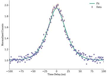
Figure 5. Experimental Autocorrelation with Fit Curve<sup>1</sup>
