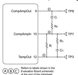
Figure 19. Feedback Loop Schematic
