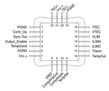
Figure 1. WTCP Pinout - Top View
