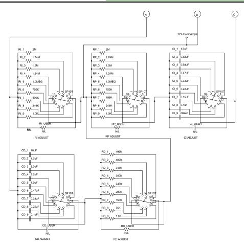
Figure 23. Schematic of P-I-D Fine-Tuning Switches
