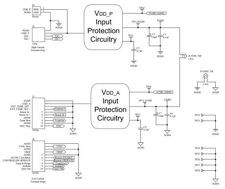
Figure 24. Schematic of Input Power Protection Circuitry
