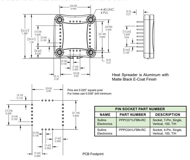
Figure 29. WTCP5V5A Dimensions
