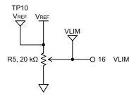
Figure 16. VLIM Resistor Divider
