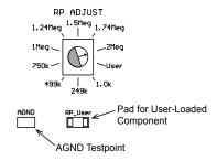
Figure 20. Feedback Switch Position
