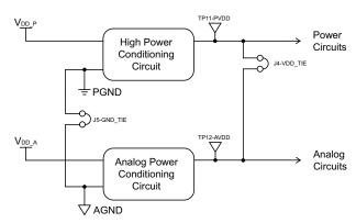
Figure 13. Power Supply Jumper Function
