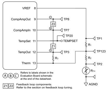
Figure 9. Temperature Control Resistor Network
