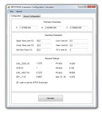
Figure 6. Configuration Calculator with Sensor Values
