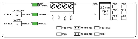
Figure 12. Power Control Section on WTCP5V5A EVAL
