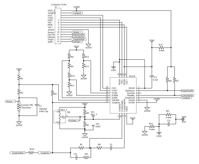
Figure 25. WTCPOEM Schematic
