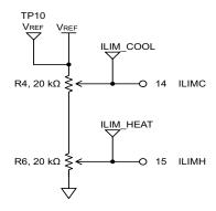
Figure 17. ILIM Resistor Circuit on Evaluation Board
