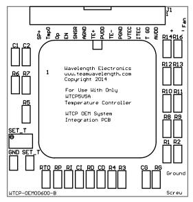
Figure 26. WTCPOEM Component Locator
