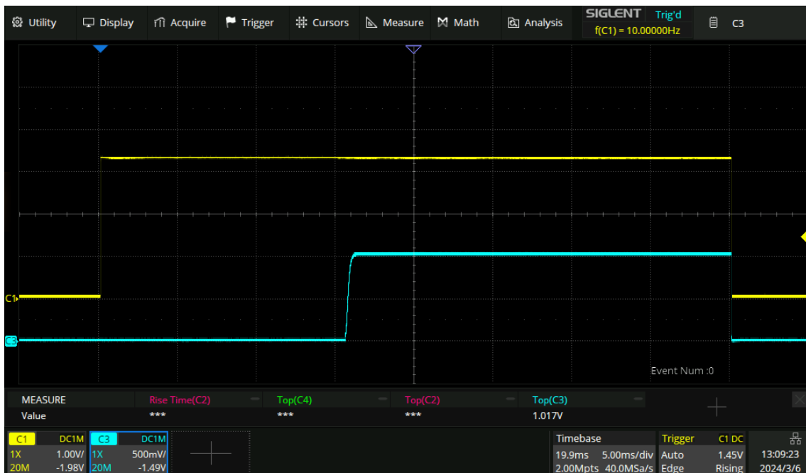
Figure 15. Current delay in control via Enable or RTO inputs. Traces: Yellow - control input, blue – output current. The current starts after ~16 ms delay.
