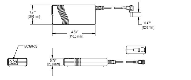
Figure 3. PWRPAK-9V & PWRPAK-12V
