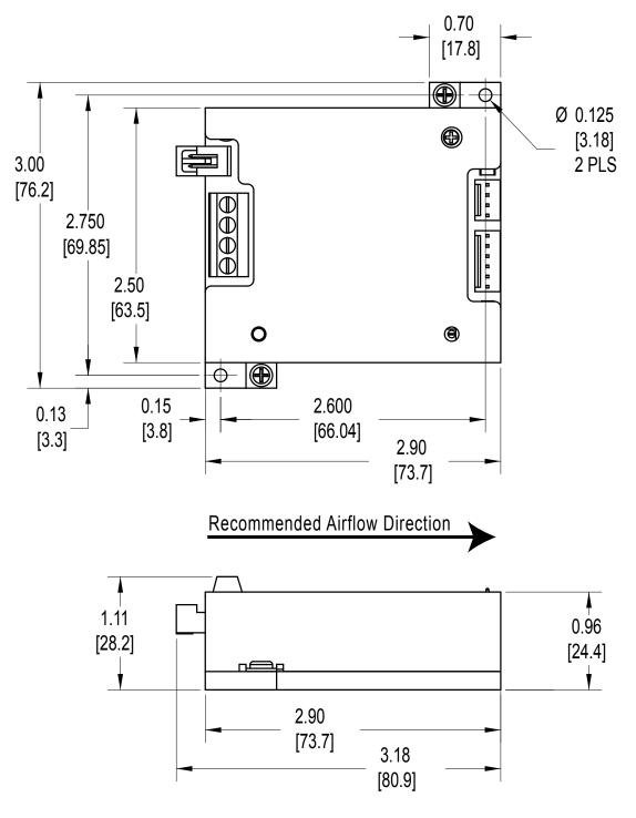
Dimensions in [mm] inches; Tolerance ±5%
