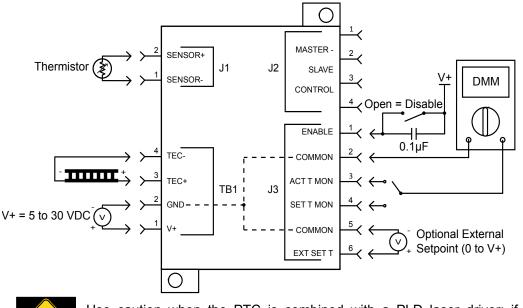
Use caution when the PTC is combined with a PLD laser driver: if the TEC or thermistor is connected to the laser diode, two power supplies may be required and must float independently of each other.
