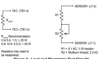
Figure 2. Load and Thermistor Test Circuits
