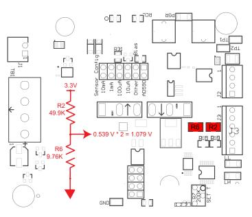
Figure 16. Safety Default Example Circuit (Rev. F)
