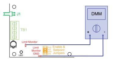
Figure 12. Monitor Test Points
