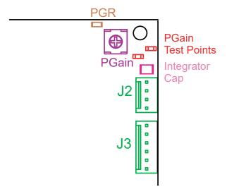
Figure 14. Proportional Gain & Test Point Locations
