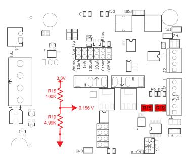
Figure 15. EXT SET T Example Circuit (Rev. F)
