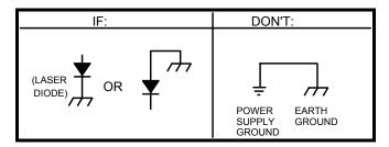
WARNING: If you plan to operate the MPL with an MPT, you may need to use separate power supplies. If the TE cooler or thermistor is connected to the laser diode, you must use two separate power supplies and let each float independent of the other.
