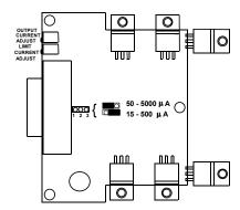
The factory set photodiode range is  $50\mu A$  -  $5000\mu A$ . As shown in the diagram above, the jumper is internal to the unit and behind the connector. To change the setting to the more sensitive range ( $15\mu A$  -  $500\mu A$ ), move the jumper to the back two pins.
