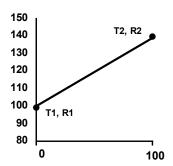
Figure 8. Typical RTD R vs. T response
