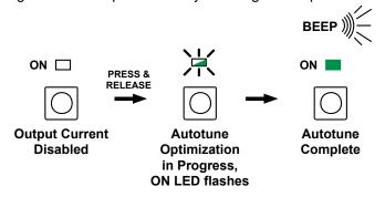
The time to complete an Autotune optimization sequence varies from load to load. While tuning, the **ON LED** will flash. When complete, the LFI will beep once and the **ON LED** will light solid.
