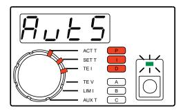
You determine what kind of control loop the Autotune will use based on your settings for the I and D terms. If set to zero, that control term will not be used. The following chart shows which control modes are available and the appropriate I and D settings. Rotate the *Display Select Switch* to I and D, making any necessary adjustments with the *Digi-Pot Adjust Knob*.
