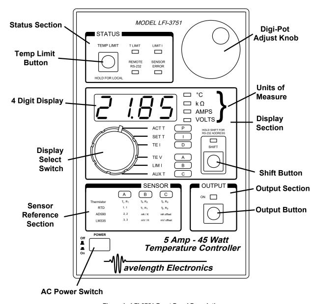
Figure 1. LFI-3751 Front Panel Description
