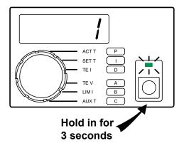
Release the **SHIFT Button** to save the displayed RS-232 address.
