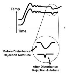
Figure 13. Disturbance Rejection Autotune Method
