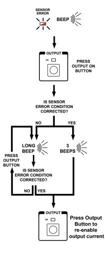
**Sensor Error LED** flashes when sensor is shorted or open. One long beep sounds if error has not been corrected after pressing the **Output Button**.
