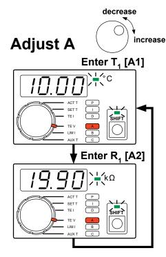
Figure 7. Entering Data Pair A - Thermistor
