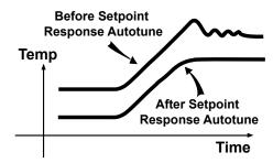
Figure 12. Setpoint Response Autotune Method
