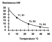
This information is available from the thermistor manufacturer (usually in table form). Use the *Digi-Pot Adjust Knob* to change either value when it is displayed. Rotate the *Display Select Switch* to **B** then **C**, making any necessary adjustments.
