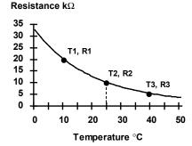
Figure 6. Typical Thermistor R vs. T Response
