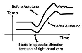
Figure 14. Non-minimum Phase System
