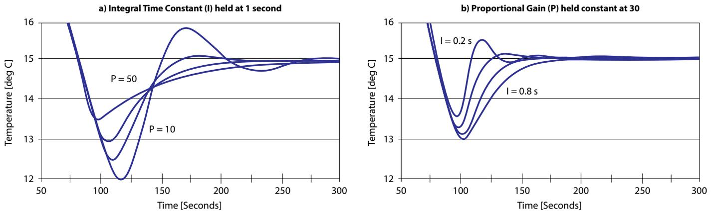
**Figure 3. Examples of trade-offs that arise when optimizing variables such as proportional gain and integral time constant.**
