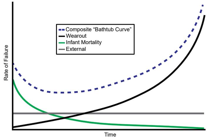
Figure 17. Laser Rate of Failure vs. Time
