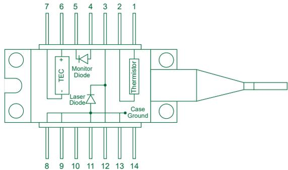
Figure 9. Standard Type 2 Laser Diode Butterfly Schematic
