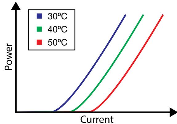
**Figure 3. Output Power vs. Input Current with Multiple Temperatures**
