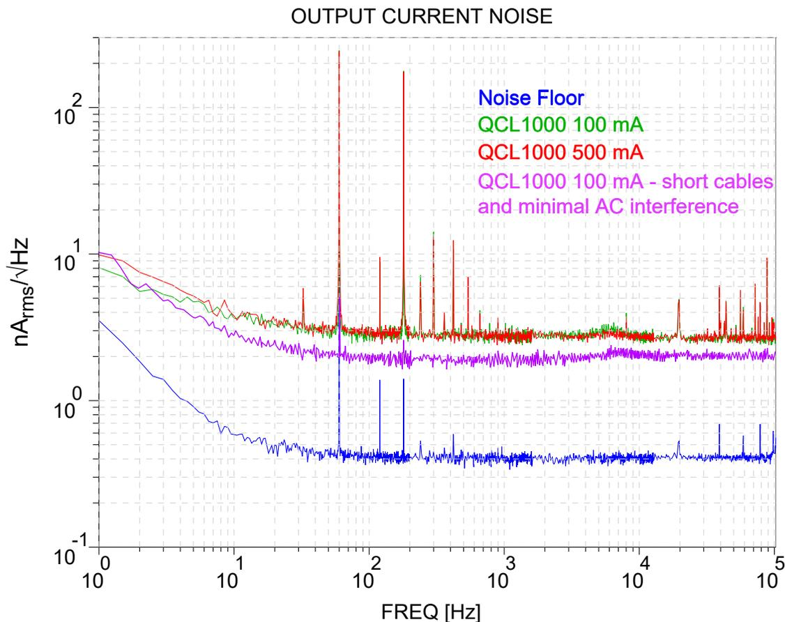
**Figure 5. Example Spectral Noise Density with long cable, AC interference, various current levels. The purple line shows an example spectral noise density with shorter cables (< 2 feet) and minimal AC interference.**
