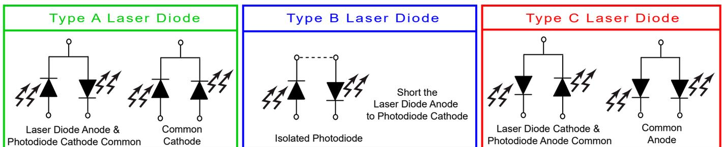
Figure 10. Laser Diode Type Diagrams
