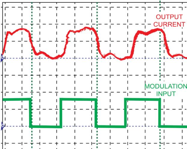
Figure 14. 20 kHz Square Wave, 4-foot twisted wires
