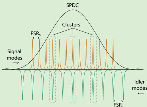
**Figure 2. Cluster effect.** The longitudinal modes for signal are shown in orange and the modes for idler are in green. The two arrows indicate the direction in which frequency increases. The overlap condition is periodical, but because of the difference in the FSRs for signal and idler, the modes that are next to the fully overlapping ones coincide only partially. This leads to a spectrum that is made of clusters of modes, separated by  $\Delta\nu_c$ .<sup>1</sup>
