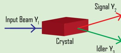
**Figure 1. Spontaneous Parametric Down-Conversion Process**
