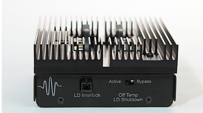
Figure 9. Interlock & Bypass side of the LDMOUNT. Interlock connection is on the left. Bypass switch is on the right.
