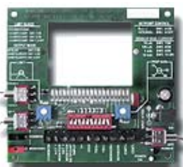
HTCEVALPCB: Evaluation Board (includes heatsink, not shown)
