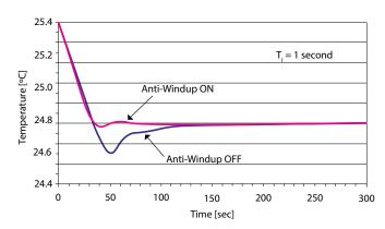
Figure 6. Comparison of response with and without antiwindup
