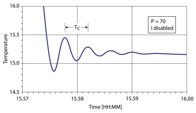
Figure 4. Find the critical proportional gain  $(k_c)$  necessary to cause the temperature to begin damped oscillations. The oscillation period is  $T_c$ .
