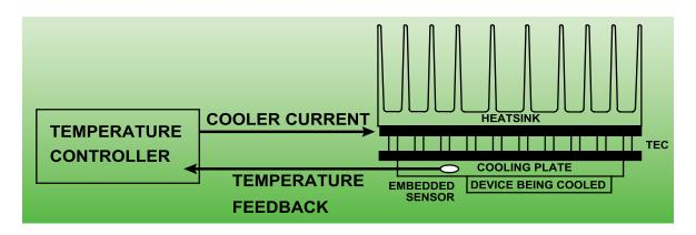
Figure 1. A simple thermoelectric control system uses feedback from a temperature sensor to maintain a device at constant temperature.
