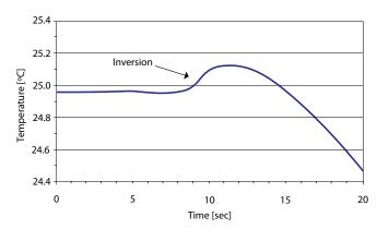
Figure 5. Inversion is the term for the system initially responding in the opposite direction from that commanded by the control signal.
