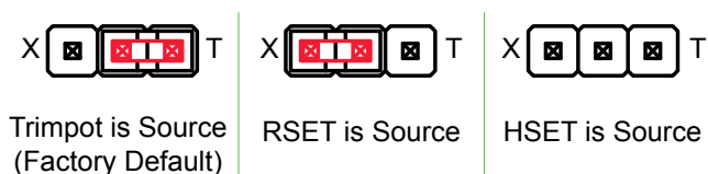
Figure 7. VSET Source Jumper Settings
