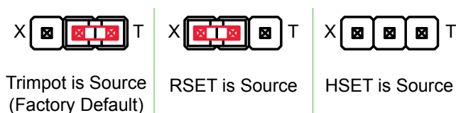
Figure 7. VSET Source Jumper Settings
